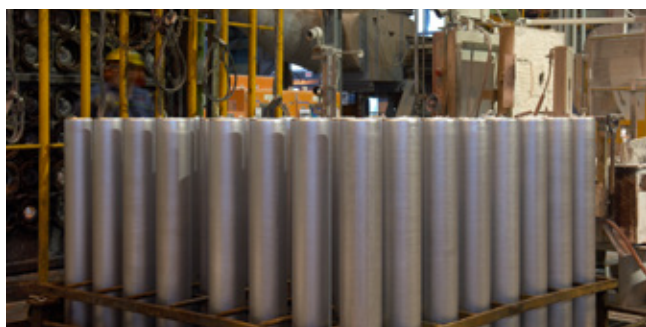
Billet ready to be lifted out of casting pit
